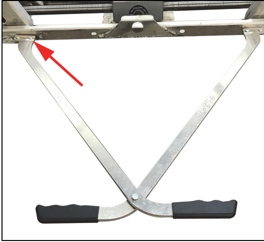
FIGURE 4. Full Car Lift Handle Installed
