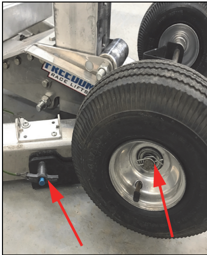
FIGURE 1. Locking Rings And Locking Pins Installed
