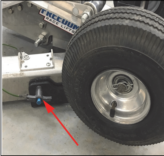
FIGURE 3. Support Arm Locking Pin Removal Location
